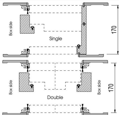
Doorpost made mainly in jointed fir veneered with ash for the lacquered ash finish, complete with antidust brush and seal.
