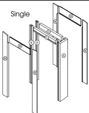
Doorpost made mainly in MDF with decorative melamine surface finish, complete with anti-dust brush and seal. The doorpost must always be cut to fit the clear opening size during installation sizes in stock for immediate delivery are always supplied with crosspieces for a 900 mm opening size, and edging trims have one larger side (3 edging trims with 30 mm projection). Both crosspieces are pre-fitted for fixing with screws with heads in the same colour.
